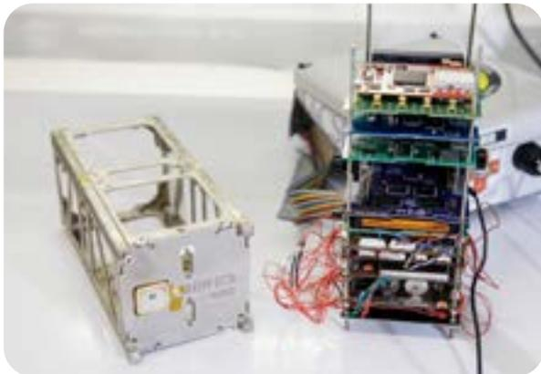
*An example satellite bus built by UNSW ACSEr that would be connected to the new Distributed FlatSat system.*
